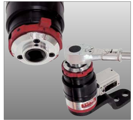
Combination of Anti-Wind-UP Clutch and Ratchet handle improves workability as well as protects operator from spring back force of the gears.
